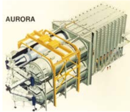
Aurora (1972–92): 50 x 50 x 100 feet, 1-1/2 million gallons of oil; 14MV and 1.6MA for 120ns. The barely visible human figures below Aurora are to scale.
